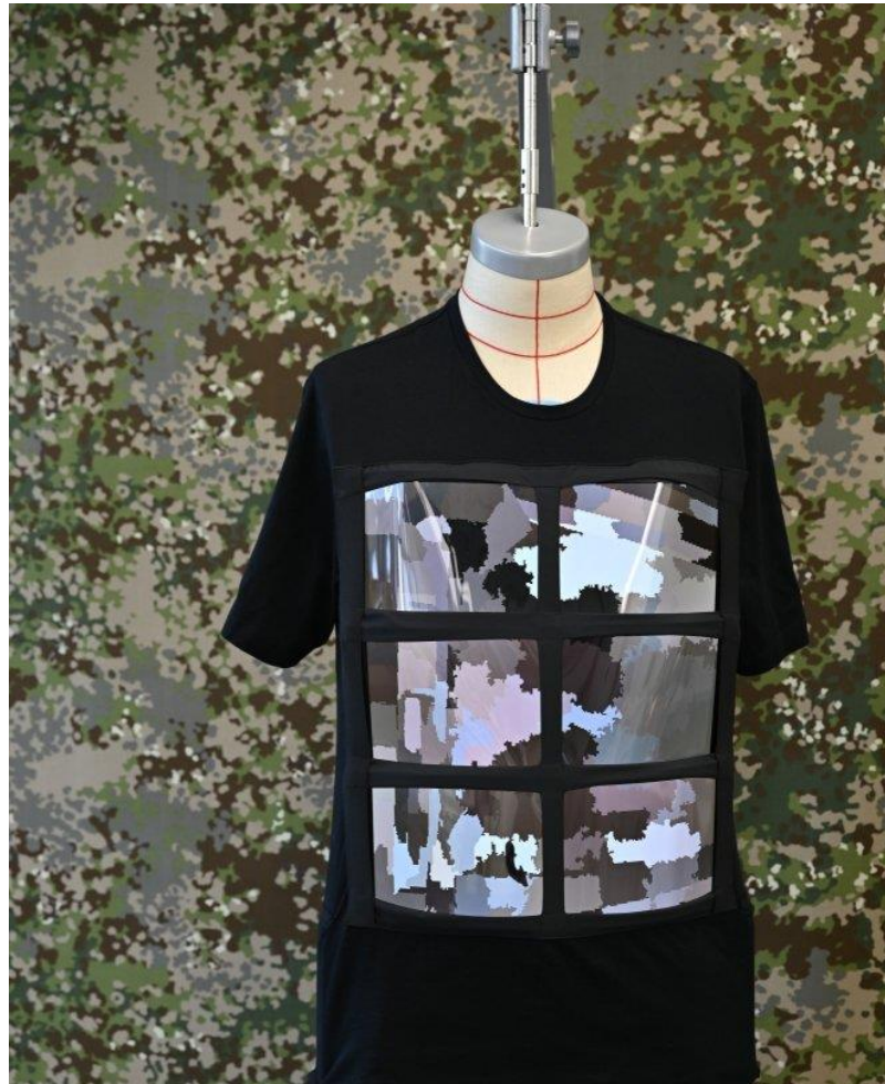
Prototype OLED-Shirt with 6 displays
