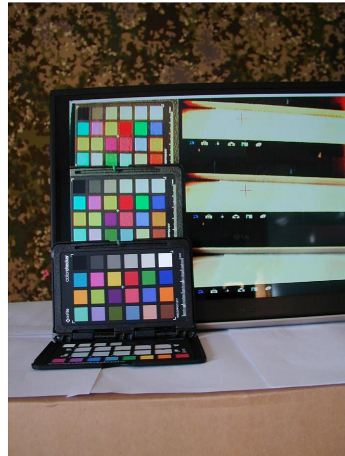
Colour reference chart in 0th, 1st and 2nd order after colour matching
