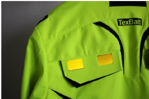
OLED on glass carrier within signal jacket [Janietz 2016]
