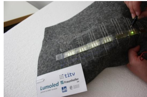
Flexible OLED-strip woven into Elitex yarn [Janietz 2016]
