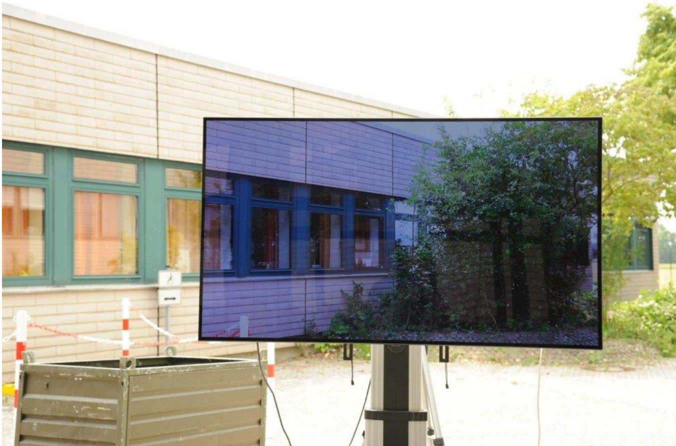
OLED Display, Company LG 55", 500 cd/m 2
