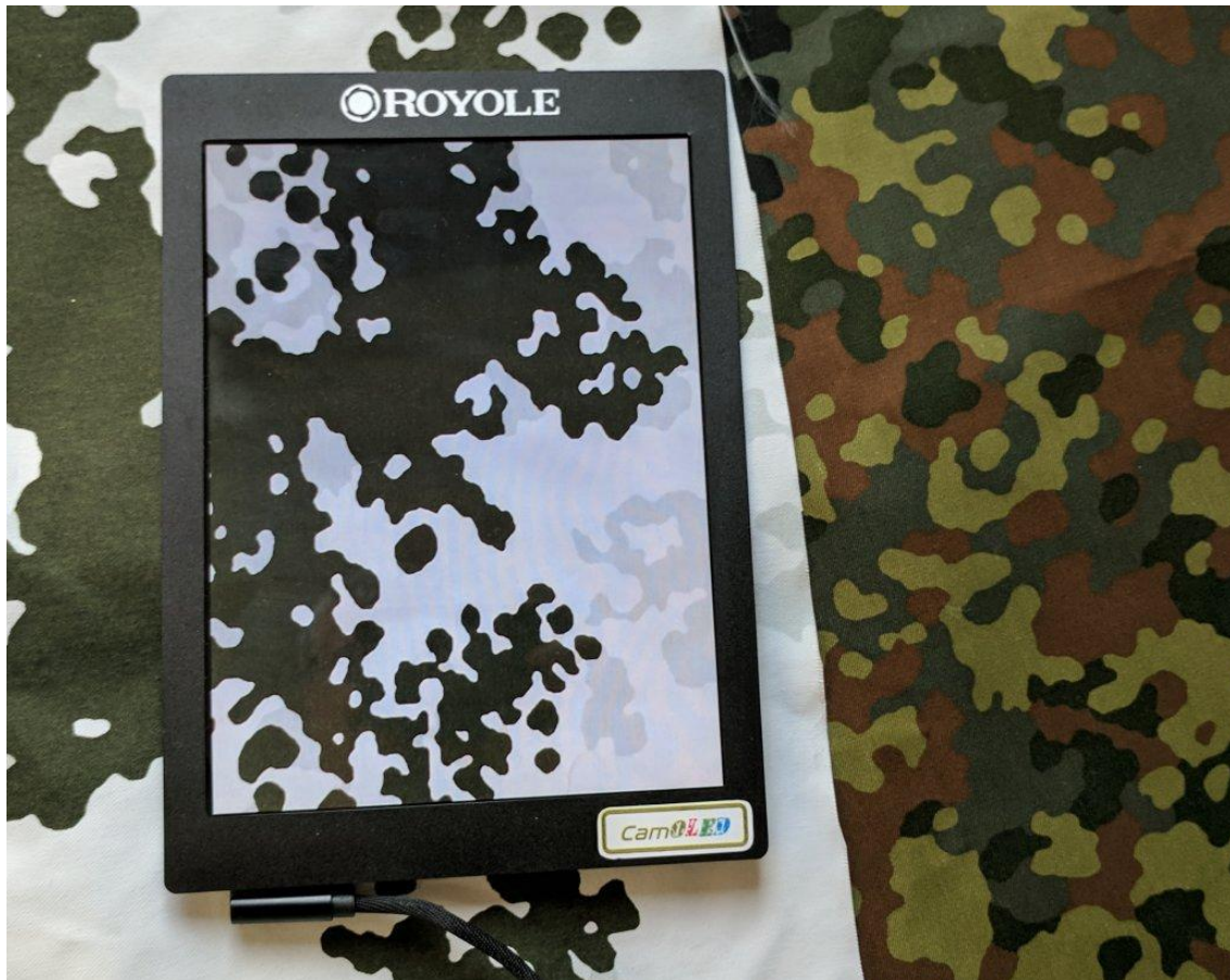
Flexible OLED display, company Royole, 140 x 190 mm 2
